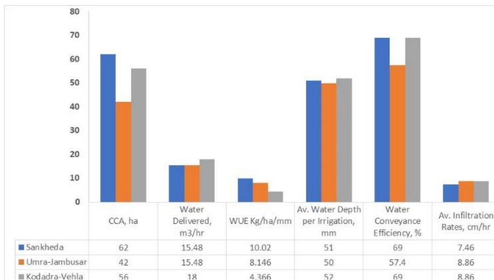
Fig. 3 Relative operational indicators observed inside sub-minors to reflect irrigation system performance
