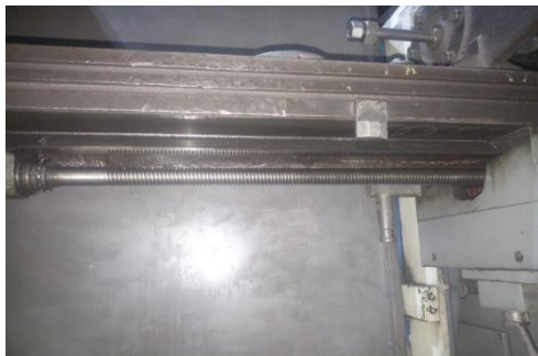
Fig. 2 – Lead screw of work table (Before)
