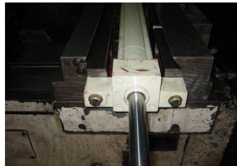
Fig. 4 –Hydraulic cylinder of work table (After)
