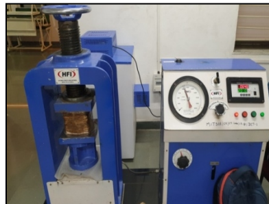
Fig. 4. Testing of cubes on CTM
