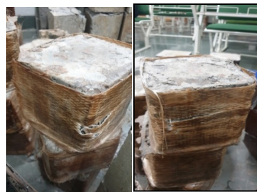
Fig.7 Fiber ruptured at face of cube and corners
