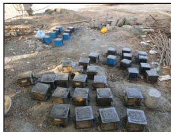
Fig. 1. Casting of cubes
