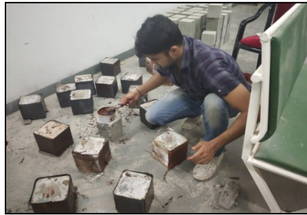
Fig. 3. Application of saturant
