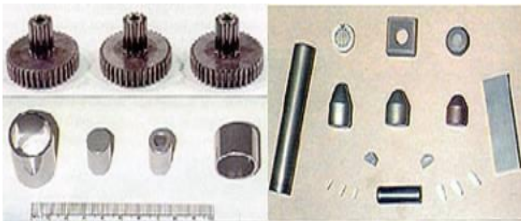
Metallic parts produced by microwave sintering such as gears cylinders, rods and discs.
