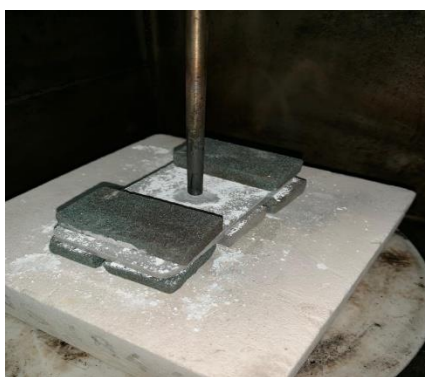
Aluminium green block in microwave furnace
