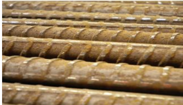
Fig 3 The "heavy" rust on the bars is tight and does not alter the deformations. The surface is acceptable & cleaning is not required.
