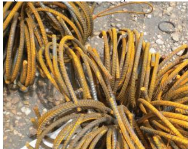
Fig 2 Although these hoops look fairly rusty, this rust is superficial and has no impact on bond behaviour.
