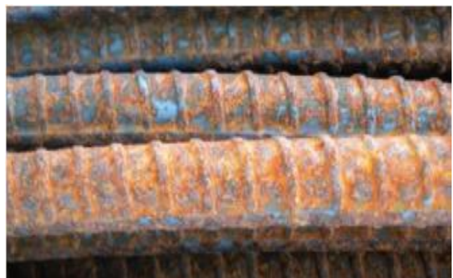
Fig 5 Close-up view of the #3 bars showing a for 20 months Tightly adhered rust pack and Good deformation definitions.
