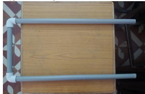
Figure: 1 Small mass Single U-Tube design of the Coriolis mass flow meter.
