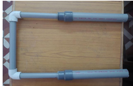
Figure: 3 The Split mass design of the Coriolis mass flow meter.
