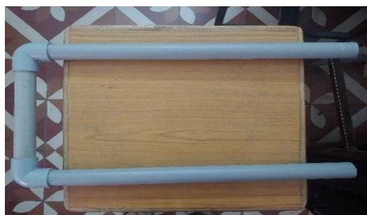
Figure: Big mass Single U-Tube design of the Coriolis mass flow meter.
