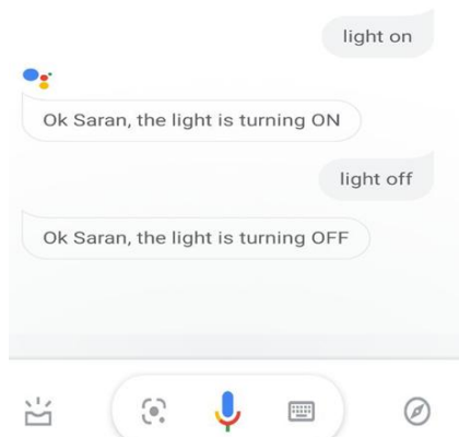
Fig:8 voice control of light using Google assistant
