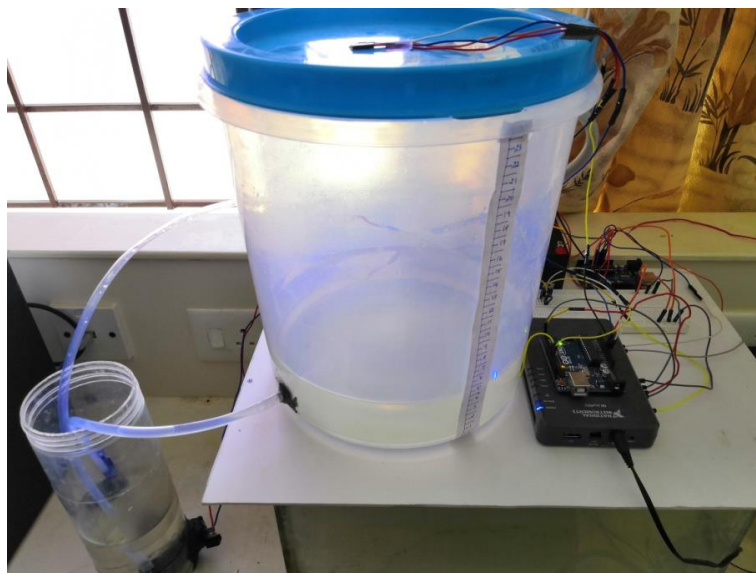
Figure 7: Experimental setup of Boiler level control
