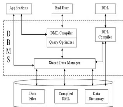
Figure. 1. Basic Model of Traditional DBMS.
