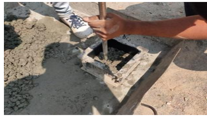
Fig. 1 Compaction of Specimen
