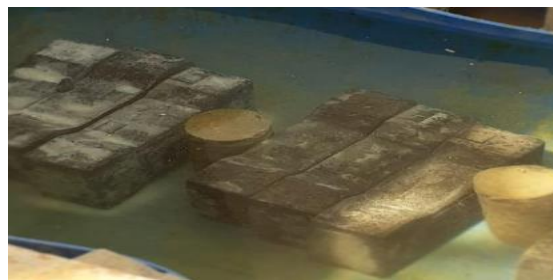
Fig. 5. Curing of specimens
