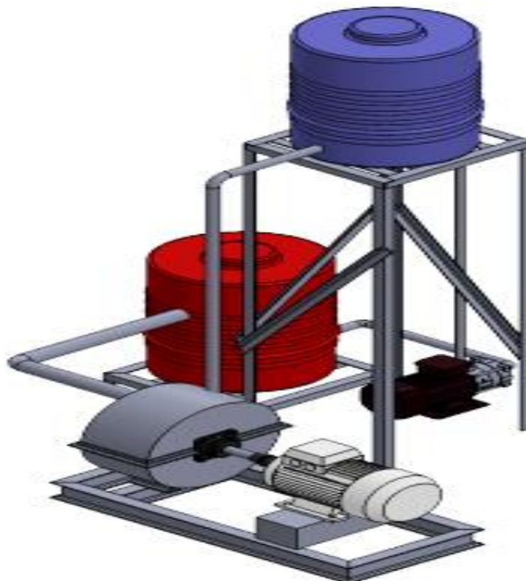
Fig. 9: Isomeric View of the Micro Water Turbine for Domestic Power Generation
