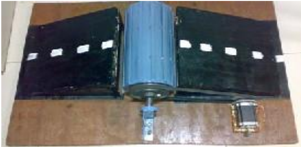
Figure 31: Rolling mechanism in speed breakers
