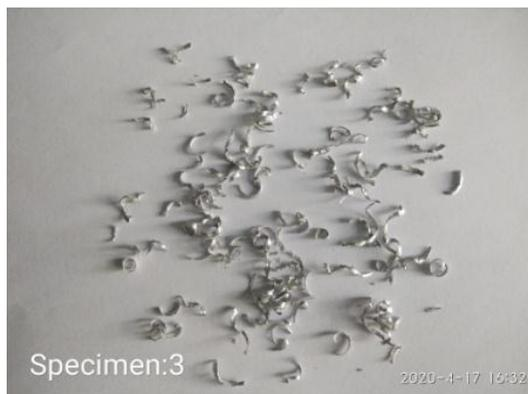
Fig.7 Chip Morphology –Specimen-3
