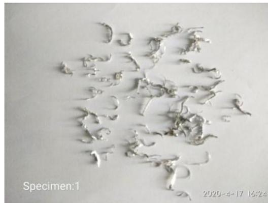
Fig.5 Chip Morphology –Specimen-1
