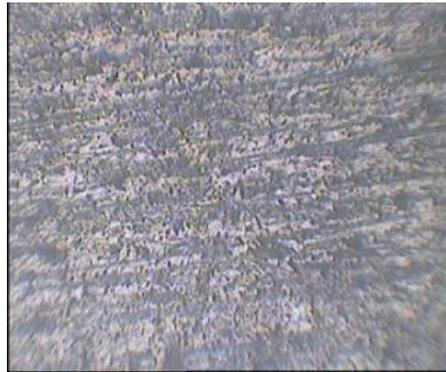
Fig.2 Al alloy without reinforcement
