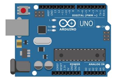
Arduino Uno is a very valuable addition in the electronics that consists of USB interface, 14 digital I/O pins, 6 analog pins, and Atmega328 microcontroller. It also supports serial communication using Tx and Rx pins. It allows the designers to control and sense the external electronic devices in the real world. The Arduino board plays important role because it consist the display module, sensor module, GSM & GPS module.
