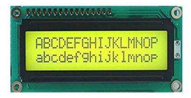
LCD (Liquid Crystal Display) is a type of flat panel display which uses liquid crystals in its primary form of operation. A display is made up of millions of pixels. The quality of a display commonly refers to the number of pixels. So display module will take input from Arduino board and display the volume of incoming fuel in the tank.
