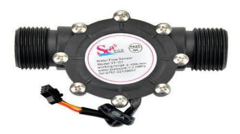
A flow meter works by measuring the amount of a liquid, gas, or steam flowing through or around the flow meter sensors. Fuel flow sensor consists of a plastic valve body, a rotor, and a hall-effect sensor. When water flows through the rotor, rotor rolls. Its speed changes with different rate of flow. Whatever the quantity measured by sensor, that value should be passed to Arduino board and Arduino board will pass that value to the display module.
