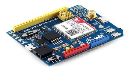
GSM module will play the important role in message passing mechanism. It will pass the message to the owner of vehicle by taking the input from Arduino board. The data of message contains quantity of fuel and total cost of fuel with respect to quantity. GPS will help for updating the location of vehicle
