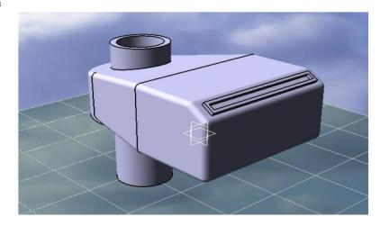
This device will measure exact quantity of incoming fuel in the tank as real time also this device will send text message to the owner of commercial vehicle with location to reduce money frauds of drives of commercial vehicle
