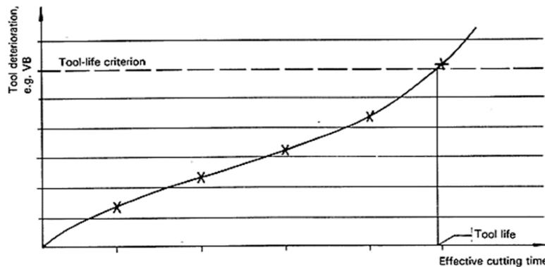
Fig.2 Tool deterioration values for a number of test runs plotted against cutting time
