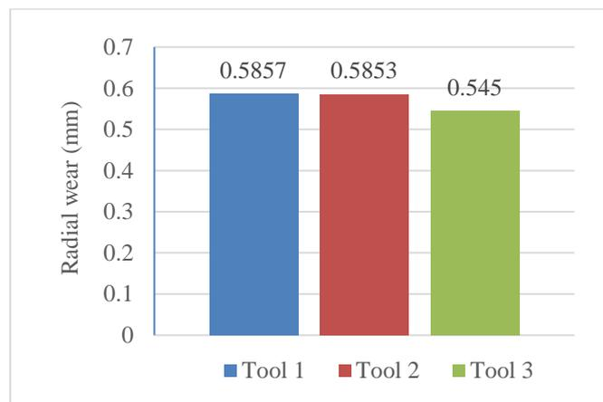
Fig. 11 Tool wear of 3 different tools used.
