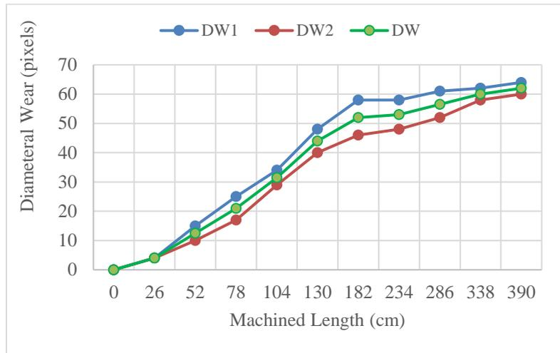
Fig. 8 Diametral Wear v/s Machined Length
