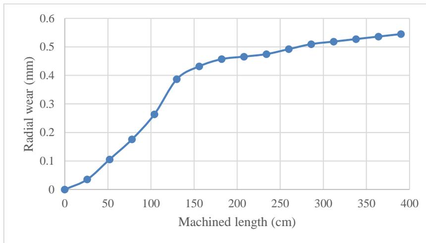
Fig. 7 Plot between Average Radial wear and machined length.
