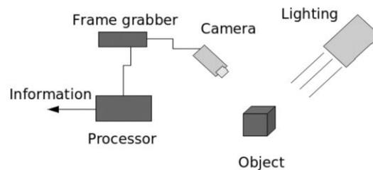
Fig. 4 General machine vision system
