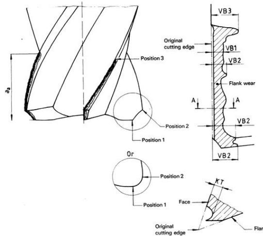
Fig.1 Wear on end mill cutter
