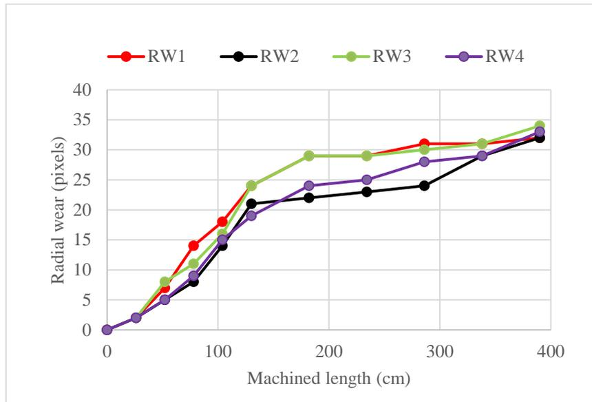
Fig. 6 Radial wear v/s Machined length
