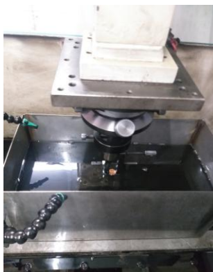
Fig. 1 Dielectric tank fitted on the EDM machine
