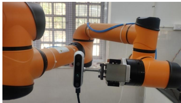
Fig.2 Eye in Hand Configuration using Aubo-i5 Robot and Intel Realsense D435 camera
