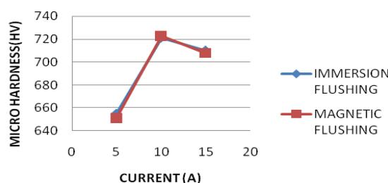
Fig 13: Effect of micro hardness on current
