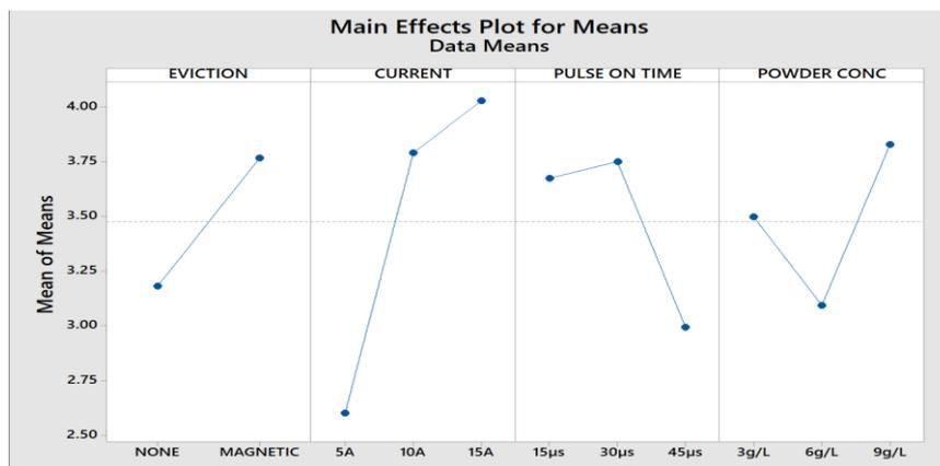
Fig 11: Effect of process parameters on SR
