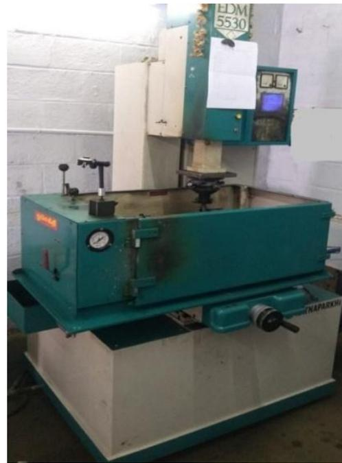
Fig 4: Die sinking EDM used in experimentation
