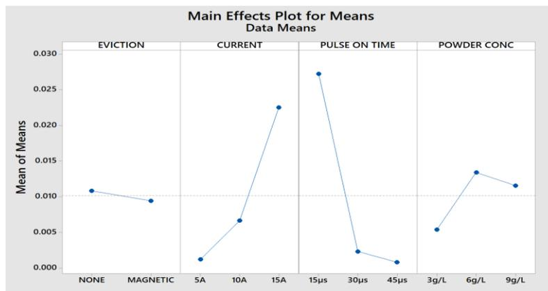
Fig 10: Effect of process parameters on TWR
