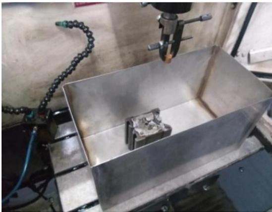
Fig 3: Arrangement of workpiece, tool and tank
