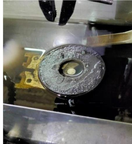
Fig 8: Magnetic debris eviction taken place in experimentation
