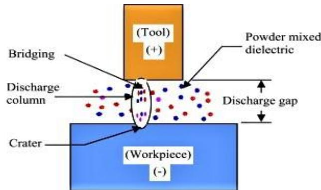
Fig. 1 Principle of Powder mixed EDM process
