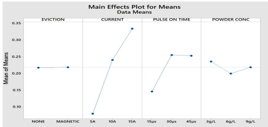
Fig 9: Effect of process parameters on MRR
