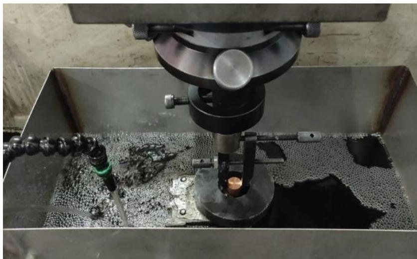
Fig 5: Magnetic flushing provided in the experimentation
