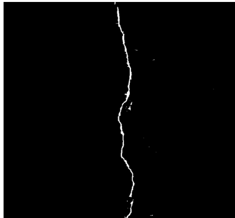
Fig 9. Area Obtained Of the Segmented Crack
