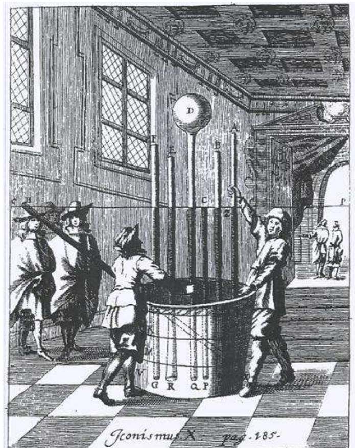
Fig.3 Large scale demonstration by Torricelli using tubes of different sizes also generated Vacuum at the top.[16]
