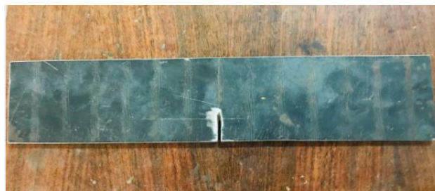
Fig 2 Steel plate with single edge crack
