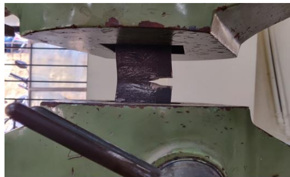
Fig 5: Deformed steel plate element
