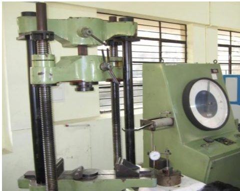
Fig 3: Experimental set up of edge cracked steel plate with uniaxial tension load
