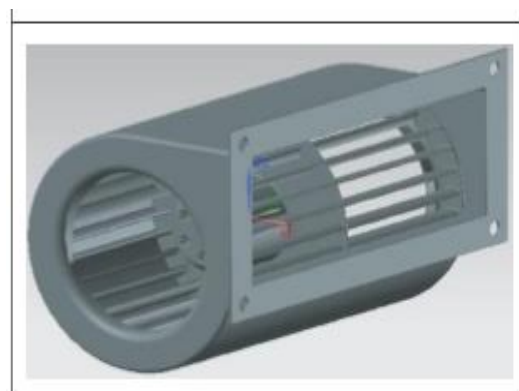
Fig.9 3D Model of the Impeller Inserted in Casing
