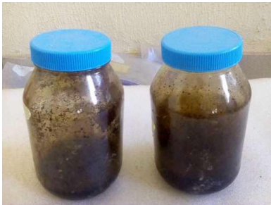
Plate 2: Sample bottles containing large deposit of Tar at temperatures below 500°C
