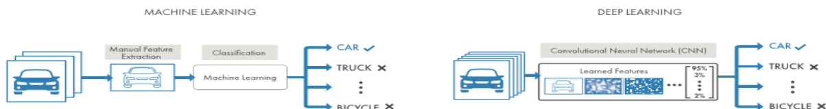
Figure 3. Comparing a machine learning approach to categorizing vehicles (left) with deep learning (right)
