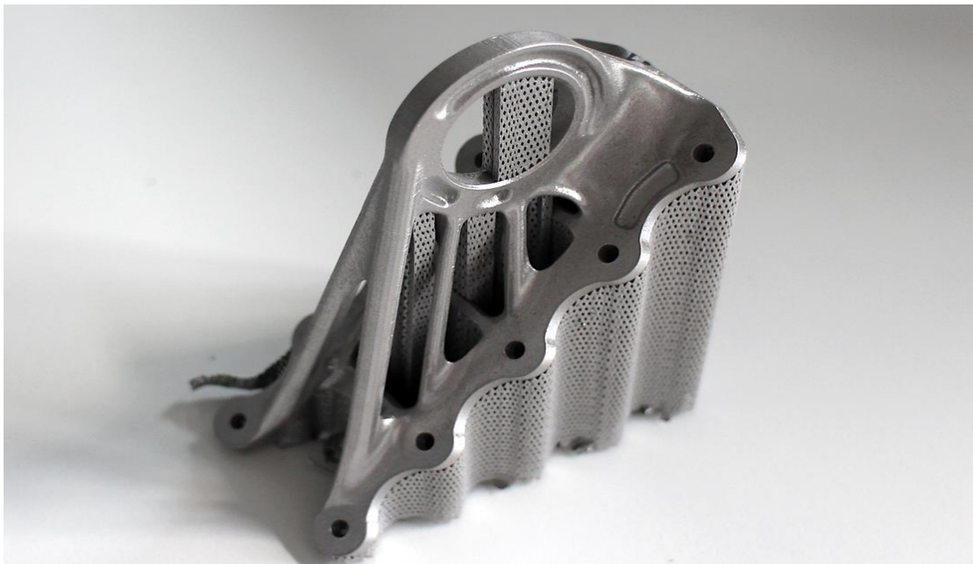
A metal bracket before support removal oriented in a 45 degree angle.
