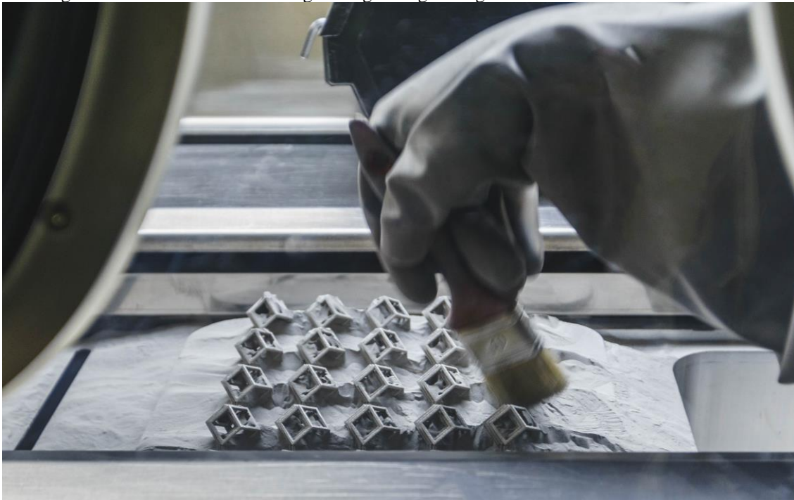
Removing the powder around metal parts produced by the SLM printing process
