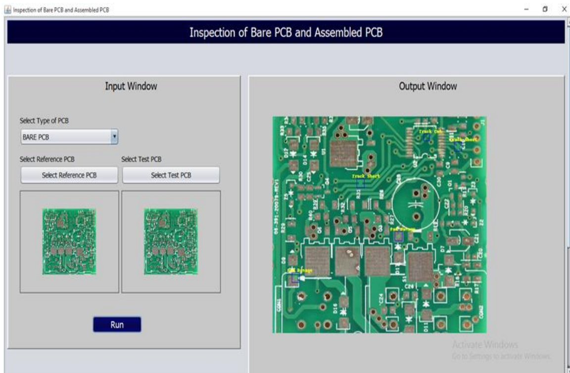
Fig. 6 Output of Bare PCB inspection in output window
