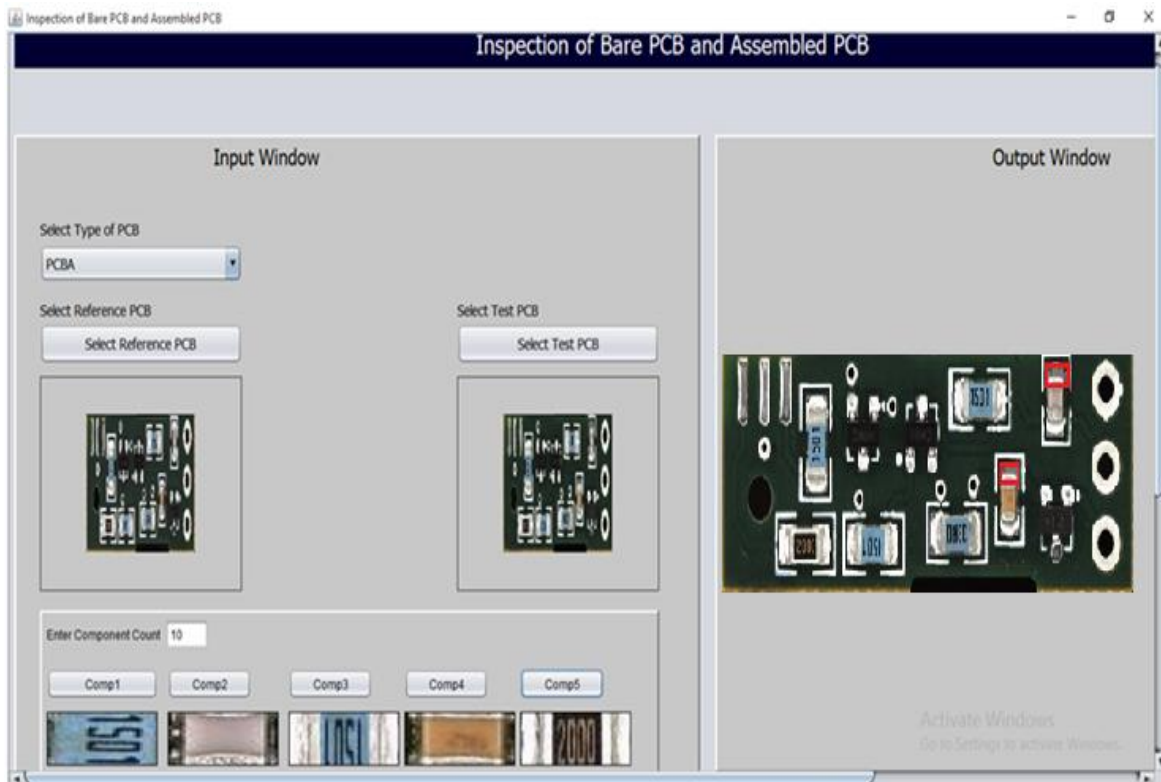
Fig. 10 The output of Assembled PCB inspection
