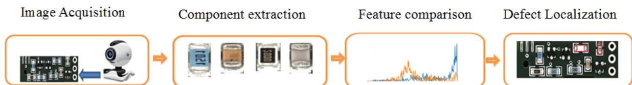
Fig. 13 Proposed Model for assembled PCB Inspection
