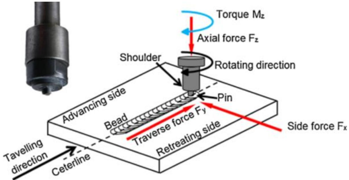
( Fig 1- Friction Stir Processing process and its tool with pin ) [34]
