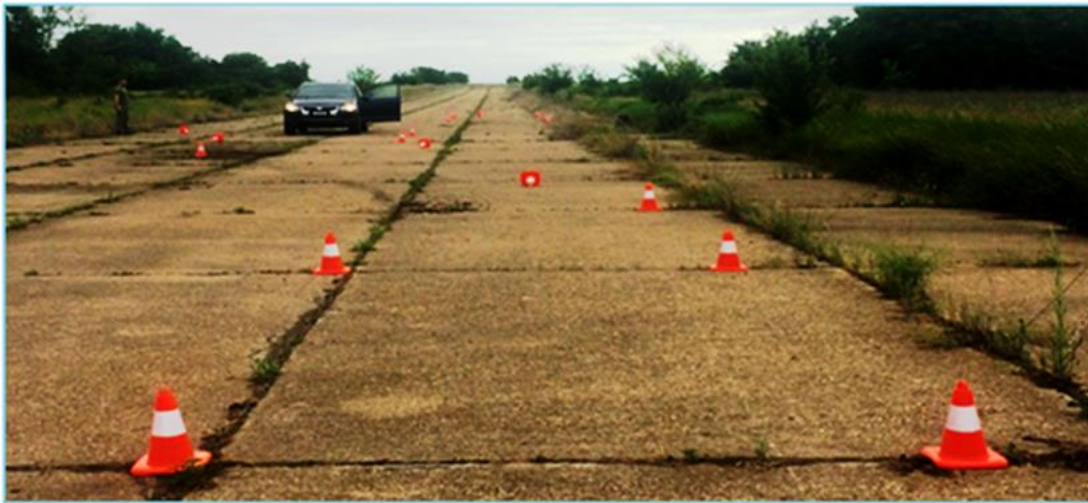
Fig. 5 Double lane change way according to ISO 3888-2
