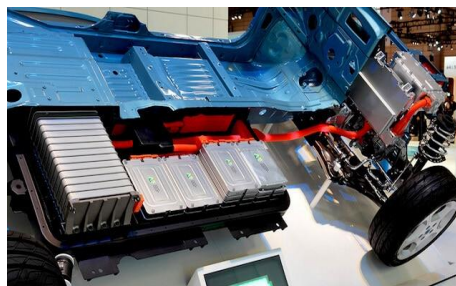
Fig 1.2 Li batteries in electric vehicle
