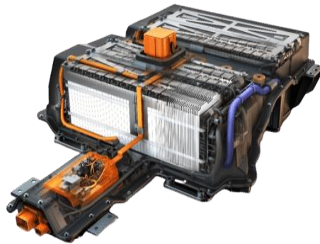
Fig 1.6 Nickel-Metal Hydride Battery Used in Electric Car
