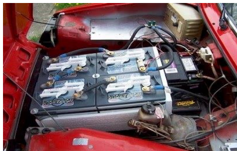
Fig 1.7 Lead Acid Battery in Electric Car
