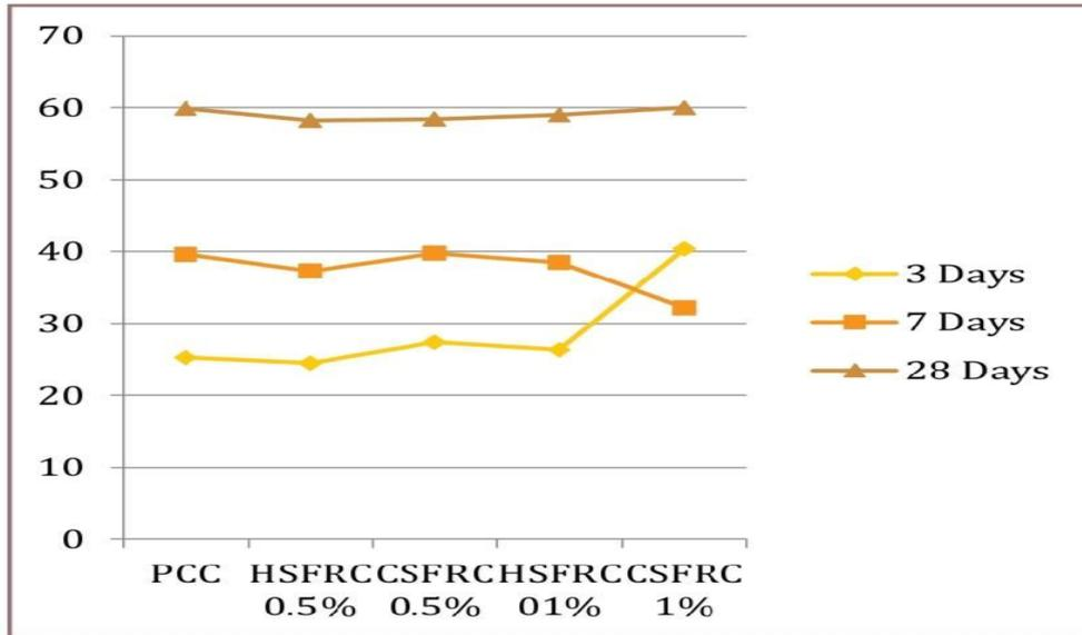
**Fig -5:** Graphical representation of compressive strength of fiber reinforced concrete
