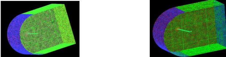
Fig 7 Illustration of unstructured mesh created on the Fluid domain and the Airfoil
