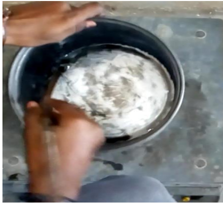
Fig 5 Mixing of Epoxy, Glass fiber and Glass Powder
