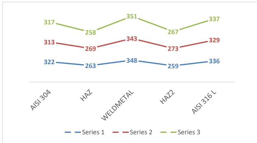
Fig. 5 Micro Hardness Chart for AISI 304 & AISI 316L at 35A
