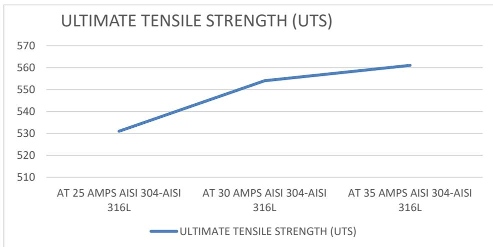
Fig. 6 Ultimate Tensile Strength at Variable amps
