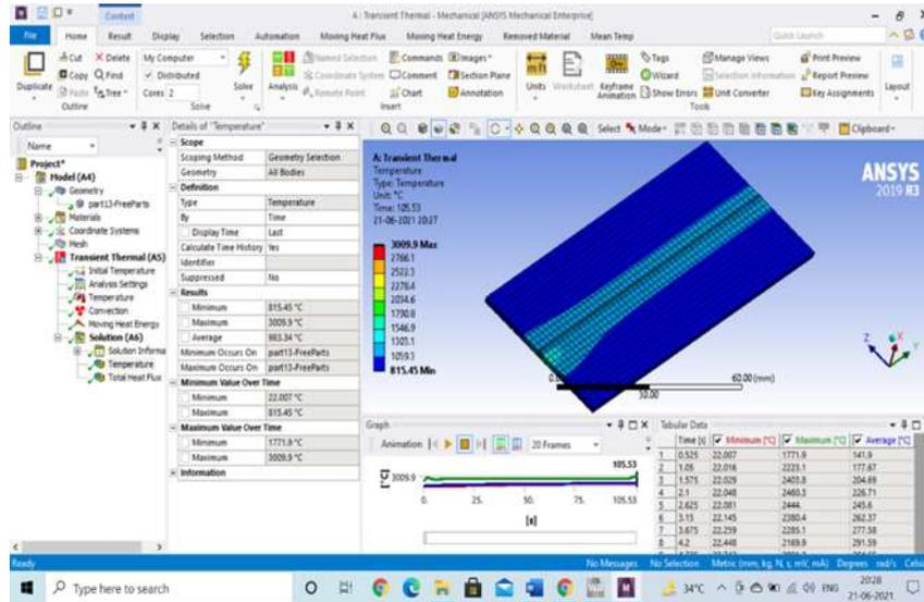
Fig. 8 Thermal Analysis of AISI 304 & AISI 316L at 25A
