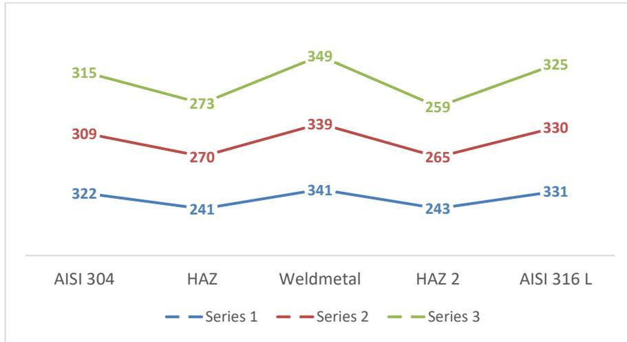
Fig. 3 Micro Hardness Chart for AISI 304 & AISI 316L at 25A
