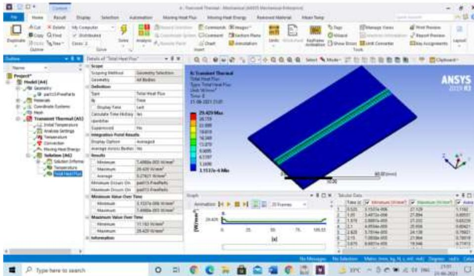
Fig. 23 Total Heat Flux Developed in AISI 304 &amp; AISI 316L at 35A
