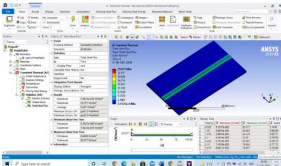
Fig. 11 Total Heat Flux Developed in AISI 304 & AISI 316L at 30A
