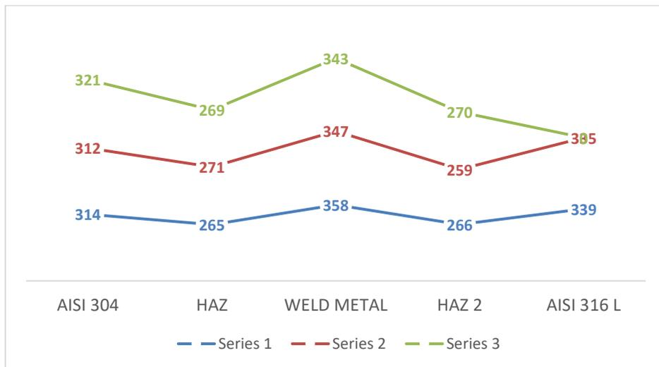
Fig. 4 Micro Hardness Chart for AISI 304 & AISI 316L at 30A
