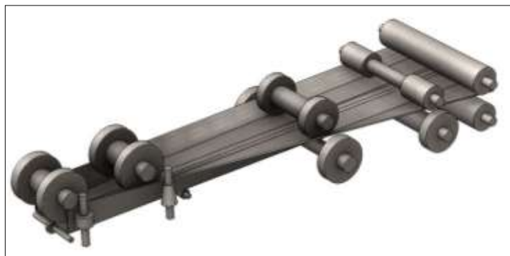
Figure 1. Roll forming process
