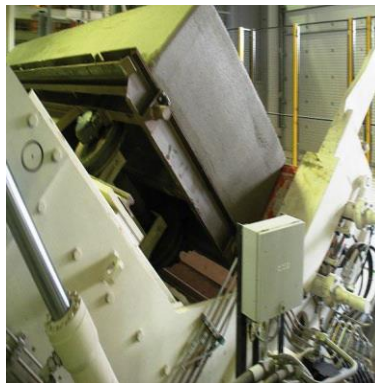
Fig. 4 Demoulding of AAC block
