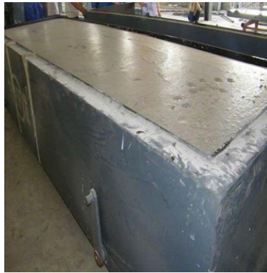
Fig. 3 AAC Blocks Casting Mould
