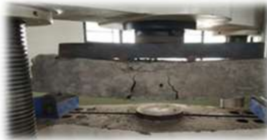
Flexural Strength Test on Beam using Universal testing Machine (UTM).
