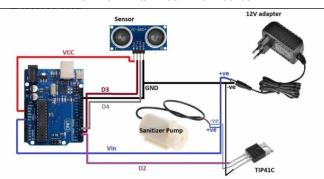
Using an ultrasonic sensor for detection of hand. So, place our hand in front of the distance sensor, it will help to the Arduino to measure the distance from the sensor to Object. The Arduino will be repeatedly sending a signal to trigger the ultrasonic sensor and when hand is present in front of the sensor then sensor will output the total time by sound to travel and from the Object then signal read by Arduino and when hand is not present in front of sensor then machine will) I turned off.
