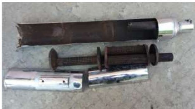
Fig.4. Cut View of Original Reflective Muffler
