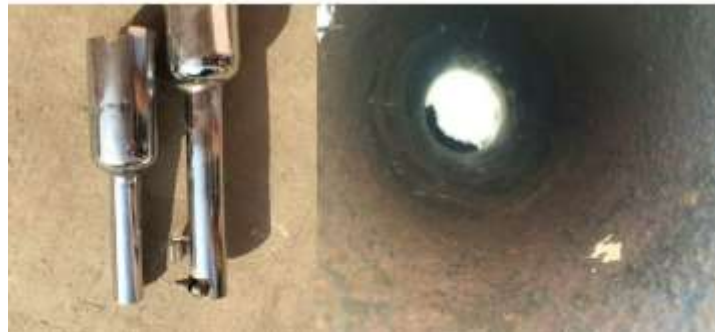
Fig.6.Cut View of Free Flow Muffler.
