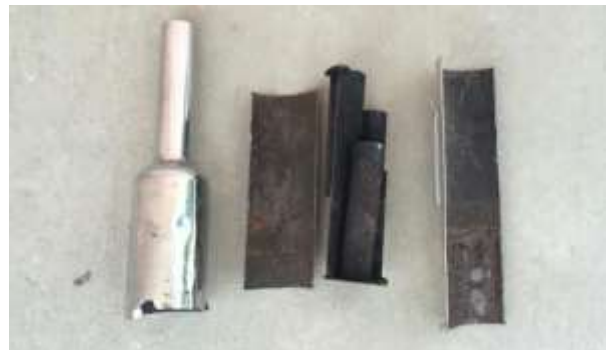
Fig.5. Cut View Of Reflective Muffler.
