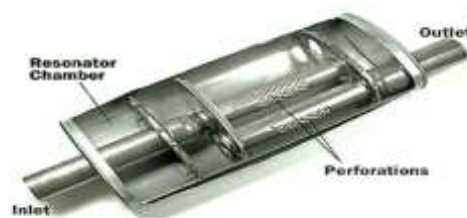
Fig.7. Cut View of Reflective Muffler.
