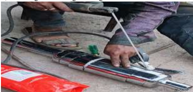
Fig.14. Welding of Cutting Parts.
