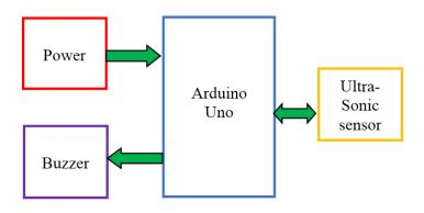
The above diagram represents the working flow of the Reverse parking sensor.
