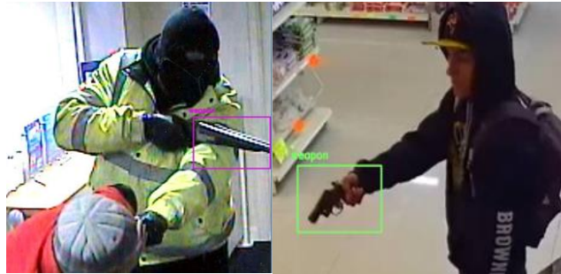
Figure 3: an example of accurate weapons detected in two different frames
