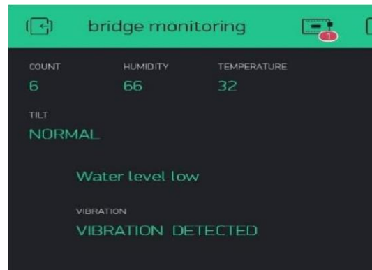
Output 3: Blynk Application showing that the water level is low and the tilt is normal
