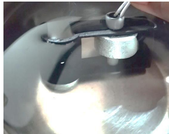
Fig 4.1.3: Sensor showing high water level increases
