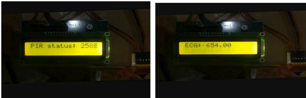
Fig .13. LCD displaying PIR Status and ECG Values
