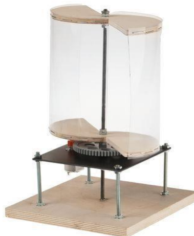
Fig:1.2 Savonius wind turbine
