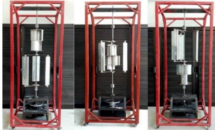
Fig1.1: Arrangements of combined Savonius & Darrieus wind turbine
