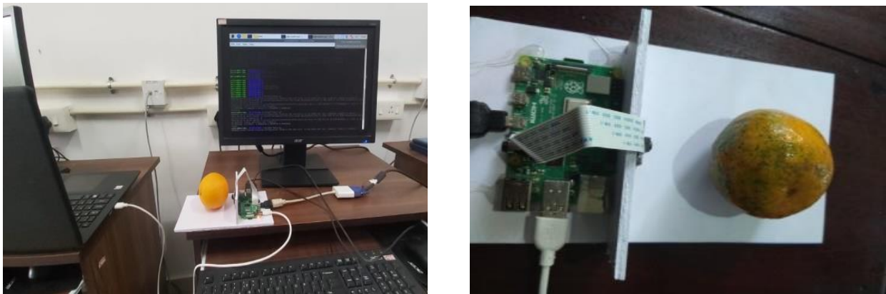
Fig 5. Raspberry Pi camera capturing image of diseased citrus(i)Canker
