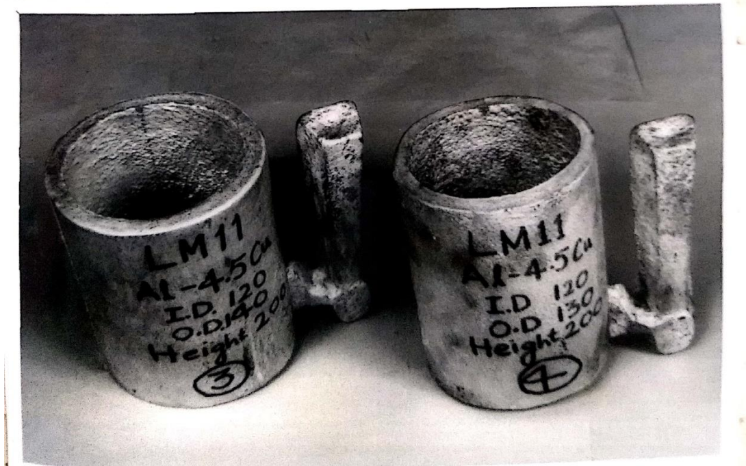
Castings of 10mm and 5mm thick and 200mm height produced without taper risers or chills.
