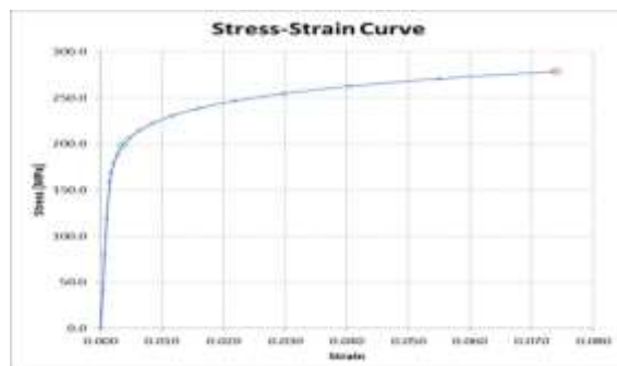
Fig 4.2 Stress-Strain curve of copper hybrid composite(C2).
