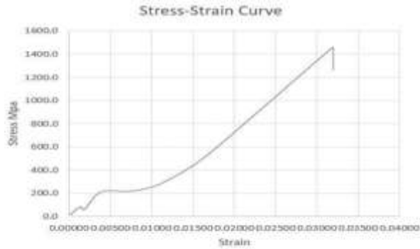
Fig 4.16. Stress-Strain curve of copper hybrid composite (C4). Fig 4.17. Stress-Strain curve of copper hybrid composite (C5)
