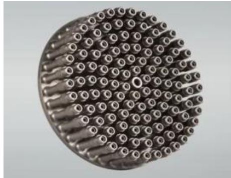
Figure 10. 3D printed injector heads [33]
