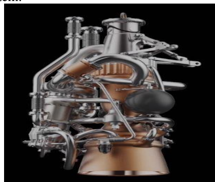
Figure 9. 3D printed liquid rocket engine [33]
