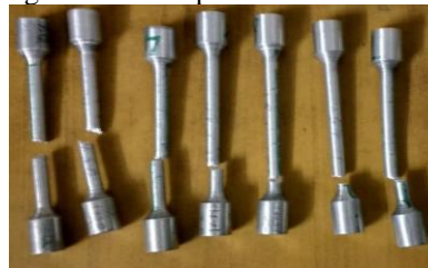
Fig. 6: Tensile Specimens after Test.
