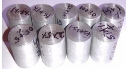
Fig. 9: Hardness Test Specimen before Testing
