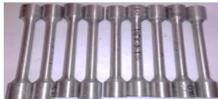
Fig. 5: Tensile Specimens before Test
