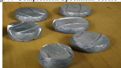
Fig. 8: Compression Specimens after Test
