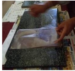
Fig 2: Hand lay-up technique process
