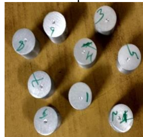
Fig. 10: Hardness Test Specimen after Testing
