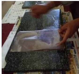
Fig 2: Hand lay-up technique process
